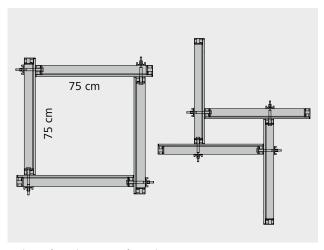
Inch-perfect shuttering for column cross-sections in 5 cm increments up to max. 75 x 75 cm side length – with few components while meeting the highest fair-faced concrete requirements.
